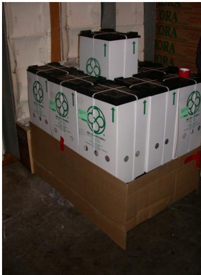
Precooling Procona boxes on a conventional horizontal pre-cooler is achieved by directing the airflow down through the boxes using an adapter plenum, and a fiberboard or fabric sleeve around the base of the boxes.
