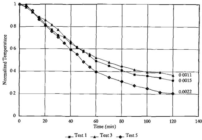
Figure 3—Normalized average temperatures from tests 1, 3, and 5 (thermocouples 1 through 6).
