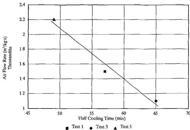
Figure 4—Comparison of air flow rate and half cooling times, tests 1, 3, and 5 ( $R^2 = 0.98$ ).
