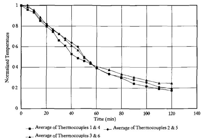
Figure 2-(c) Test 5 - Forced-air, normalized temperatures (thermocouples 1 through 6).
