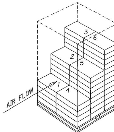
Figure 1—Location of thermocouples in pallet of fruit.
