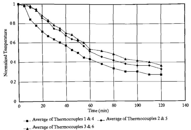
Figure 2-(a) Test 1 - Forced-air, normalized temperatures (thermocouples 1 through 6).
