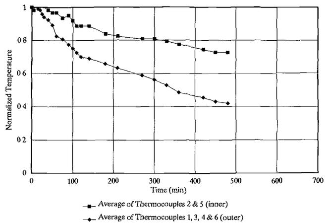
Figure 5—(a) Test 2 – Room cooling, normalized and averaged temperatures.
