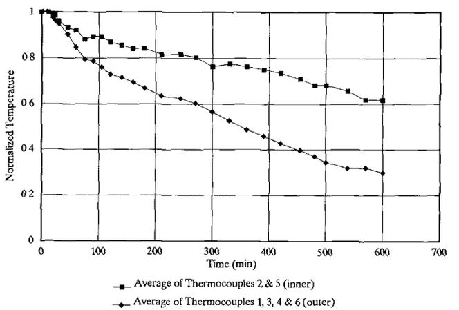
Figure 5—(c) Test 6 – Room cooling, normalized and averaged temperatures.
