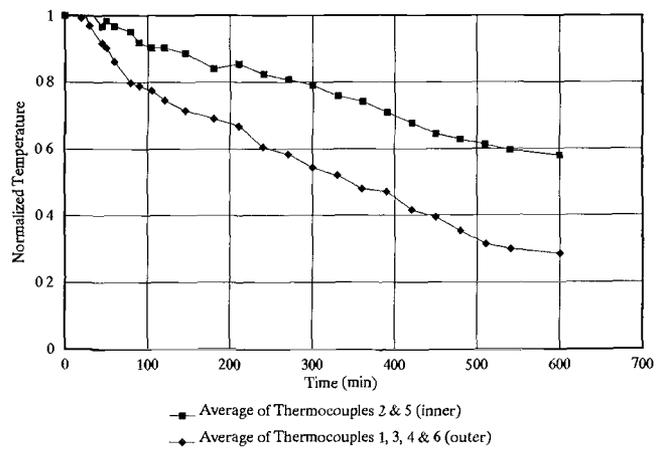
Figure 5—(b) Test 4 – Room cooling, normalized and averaged temperatures.
