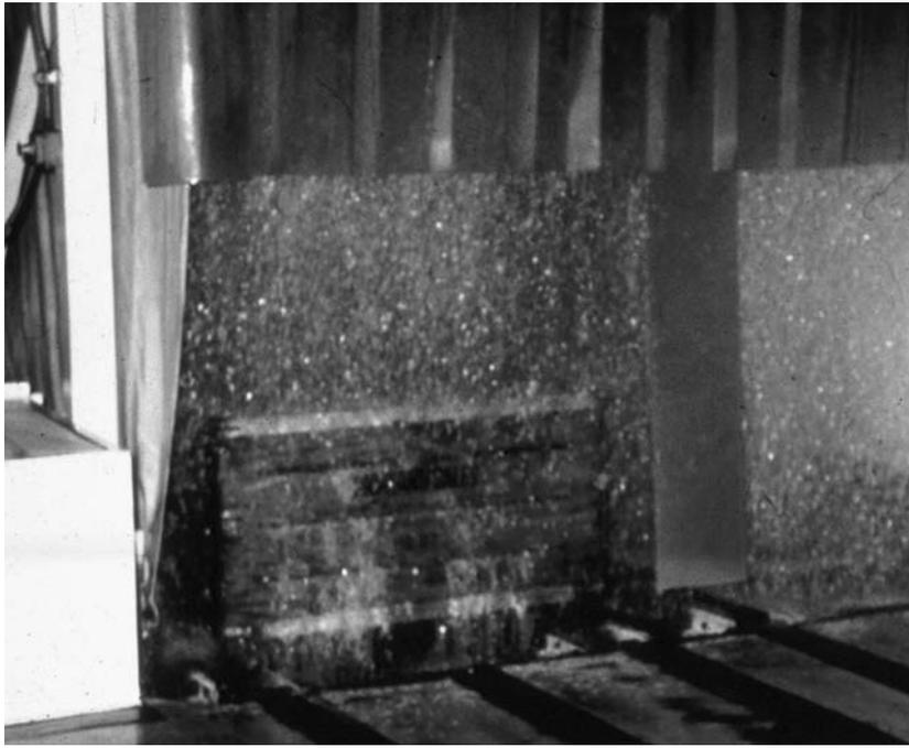
Fig. 22.3. Bin of peaches being pre-cooled on a conveyor-type hydro-cooler prior to packing.
