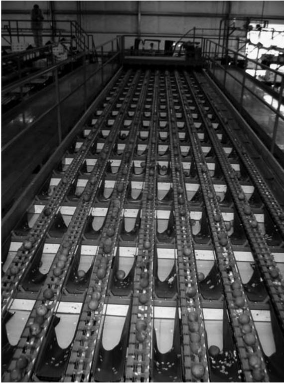
**Fig. 22.12.** Fruit moving on to an electronic weight sizer.
