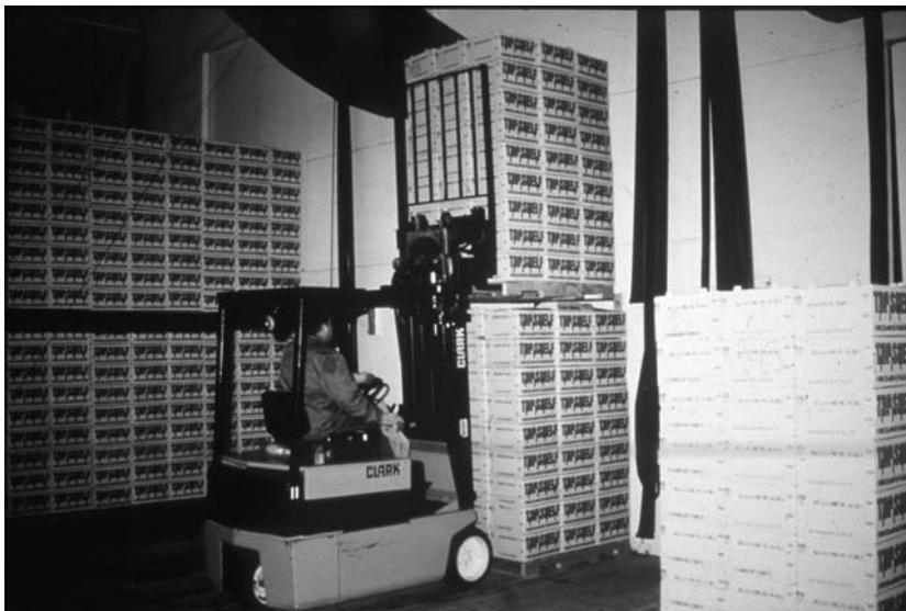
Fig. 22.4. Packaged fruit in unitized pallet loads are stacked to form a forced-air cooling tunnel.
