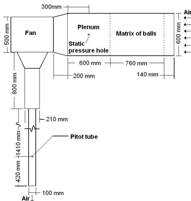
**Figure 2.** Top view of the experimental set-up.
