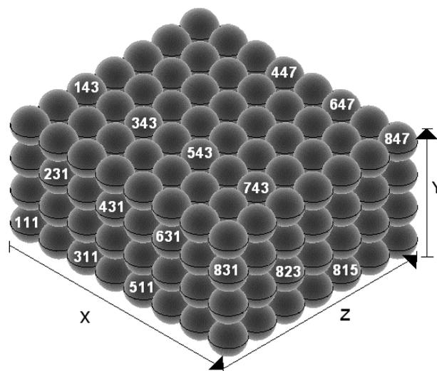
**Figure 1.** Overview of the matrix of balls. The numbered balls are instrumented. The three digit number on a ball represents the X, Y, and Z positions, respectively.
