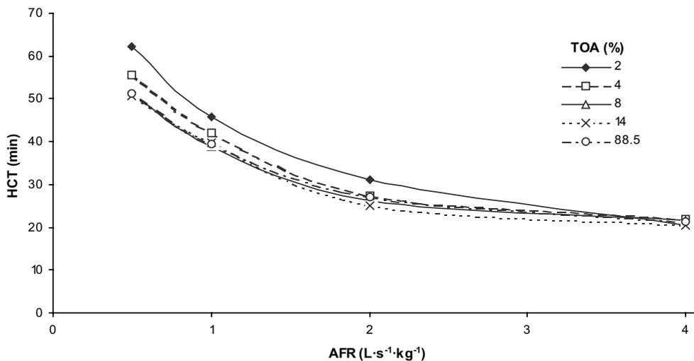
Figure 3. Half-cooling time (HCT) as a function of airflow rate (AFR) and total opening area (TOA).
