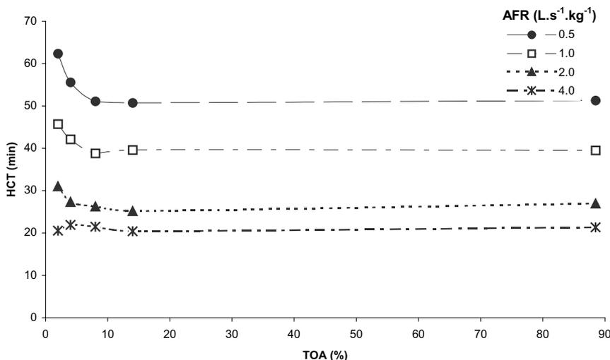
Figure 4. Half-cooling time (HCT) as a function of total opening area (TOA) and airflow rate (AFR).
